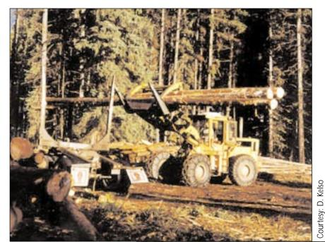
A front-end loader is used to load logs onto a logging truck.
